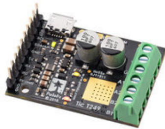
Tic T249 USB Multi-Interface Stepper Motor Controller (Connectors Soldered).
