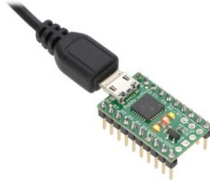
The P-Star 25K50 Micro with soldered headers and connected USB cable.
