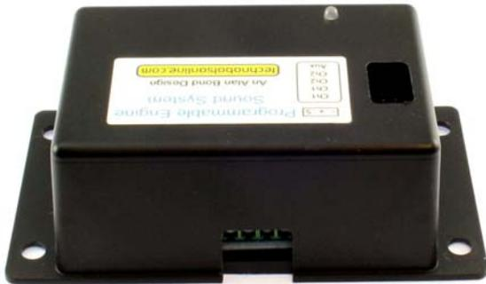
The receiver channel and ESC leads may be connected through the aperture in the top of the box, taking care to observe the polarity marking on the label – this means the black lead to the edge of the box and the white (or sometimes orange) lead to the centre of the box.
