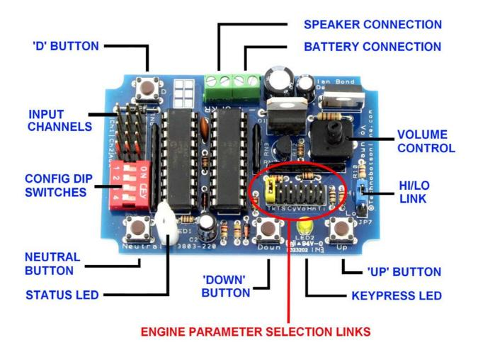
Make connections to the Sound System (as described later), configure it and try it out with the case removed. Make sure the Sound System is not placed on a metallic surface or surface contaminated with metal debris, placing it on the base plate is recommended.
