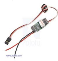
A typical commercial 5V BEC is shown here, which can drop the typical 12V speaker supply down to the requisite avoiding the 5V. thus logistics accommodating and charging an extra set batteries with the benefit that the main power switch will also switch off the 5V output from this unit. It also benefits from being supplied with a standard RC lead/plug which is directly compatible with the Sound System. The unit shown is Technobots part 1062-017
