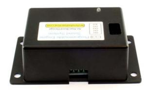
The control potentiometer and push button leads may be connected through the aperture in the top of the box, taking care to observe the polarity marking on the label – this means the black lead to the edge of the box and the white (or sometimes orange) lead to the centre of the box.
