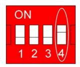
This is the **POTENTIOMETER CONTROL** version of the manual. Before proceeding further, check that switch 4 of the configuration option switches is set to the ON position to configure the unit for **POTENTIOMETER CONTROL**.
