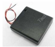
A battery pack can be made up using 4 AA cells in a suitable holder – preferably a type that is both enclosed and switched, such as Technobots part 1063-063. Either re-chargeable NiMh or primary (single use) cells may be used – the former yielding a nominal 4.8V (1.2V per cell) or the latter yielding 6v (1.5V per cell) due to the different battery chemistries involved.
