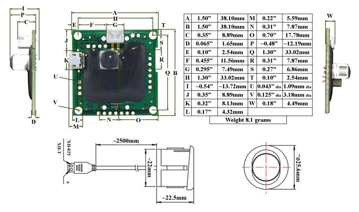
The recommended operating and storage temperature of the MB8450 Car Detection Sensor is -40C to +75C.
