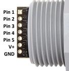
**Pin 3- Analog Voltage Output:** After the ~50ms power up initialization, the voltage on this pin is set to 0V. Once the sensor receives a range value the voltage on this pin has the voltage corresponding to the latest measured distance. This pin outputs an analog voltage scaled representation of the distance.
