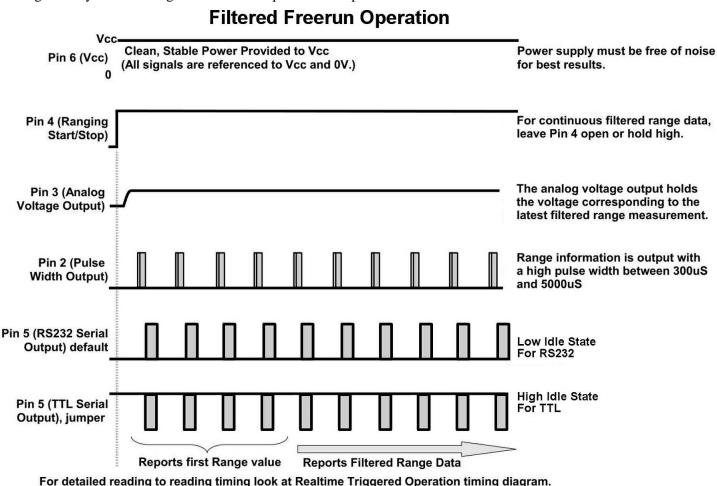
When pin 4 is left high, the sensor will continue to range every 133mS (7.5Hz read rate), the data output includes a 1.5Hz filter. The HRXL-MaxSonar-WR sensors will output the range based on recent range information. The filter does not affect the speed at which data is made available to the user but instead allows for more consistent range information to be presented.
