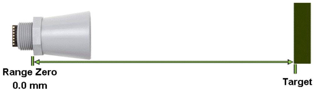
The range is measured from where the housing meets the threading.
