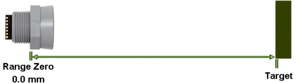
The range is measured from where the housing meets the threading.
