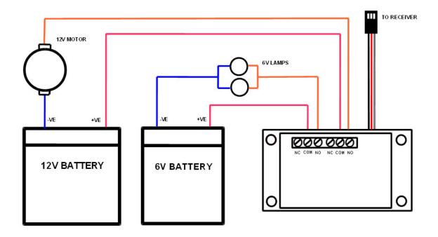
The following diagram illustrates how the unit may be connected up to give simple bi-directional control of a motor, including stop. Both switches should be configured in non-latching (momentary) mode for this application.
