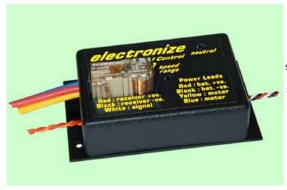
The electronic control plugs directly into the 'throttle' output of the receiver with no need for a servo. There is no need to match the electronic control to the motor other than to stay within the maximum ratings. The same control will work equally well with a large or small motor.
