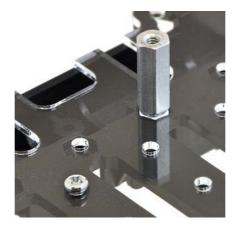
The mounting plate is secured to the chassis with screws through the two rounded tabs that protrude from the front edge, along with any number of the interior-nut mounting holes in the rear.
