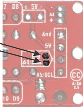
The SMD LEDs on the bottom of the SMD-versions of the BackPack can be each (or globally) disabled by cutting the trace connected to the LED just above each of the “Dx” labels.
