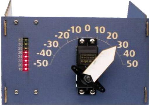
Dual-Temperature display using Ardweeny Backpack's Servo-output, LED bargraph, and TMP36 temperature sensor. Get source-code from our website!
