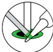
**Do:** While continuing to hold the iron in contact with the leg and metal ring, feed solder into the joint.
