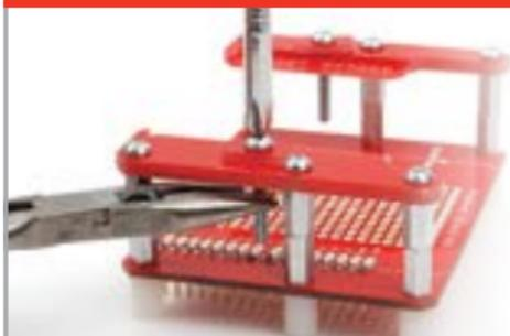
It's tricky to adequately tighten the locknut with your fingers. Holding the nut with a pair of needle-nose pliers will save time and frustration.
