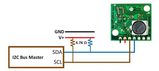
The four minimum required connections to the sensor to obtain basic functionality are: ground and power to GND and V+ respectively, SCL to Pin 5, and SDA to Pin 4.
