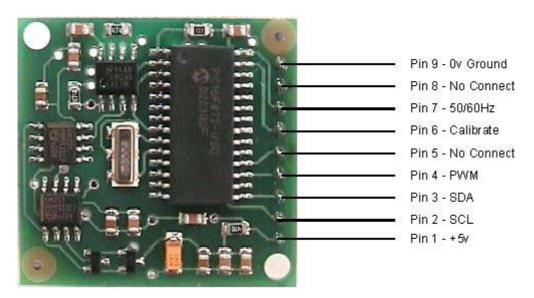
The compass module requires a 5v power supply at a nominal 15mA.
