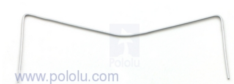
The middle legs of the hexapod. The segments at the end should be 1.25" in length.
