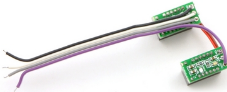
Soldering the sensors to a four-pin cable.
