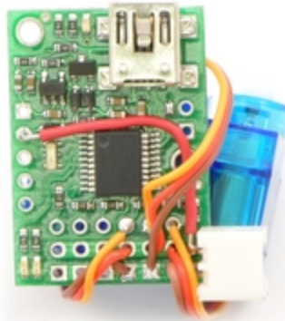
Connecting the servos to ports 0, 1, and 2 on the Micro Maestro.
