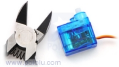
A sub-micro servo with mounting tabs clipped off.
