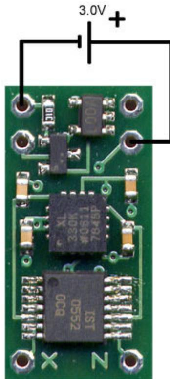
This would be useful for e.g. an application powered directly by 2 AA batteries or a lithium coin battery. The minimum operating voltage when using bypass mode is  $2.0\text{V}$  and **the absolute maximum voltage that can be applied when bypassing the regulator is  $3.6\text{V}$ .**
