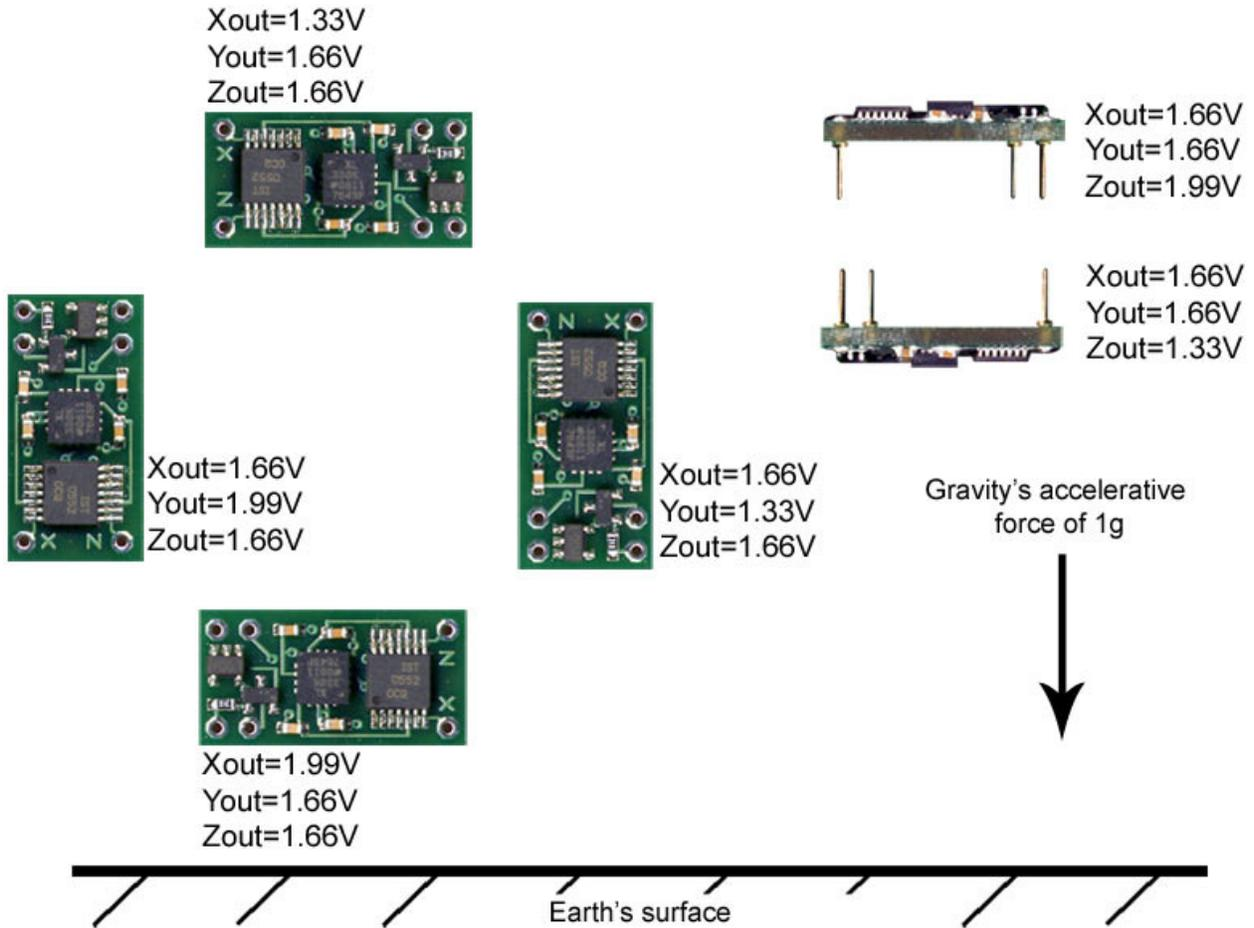
The voltage outputs on the DE-ACCM3D correspond to acceleration being experienced in the X, Y and Z directions. The output is ratiometric, so the output sensitivity (in mV/g) will depend on the supply voltage.
