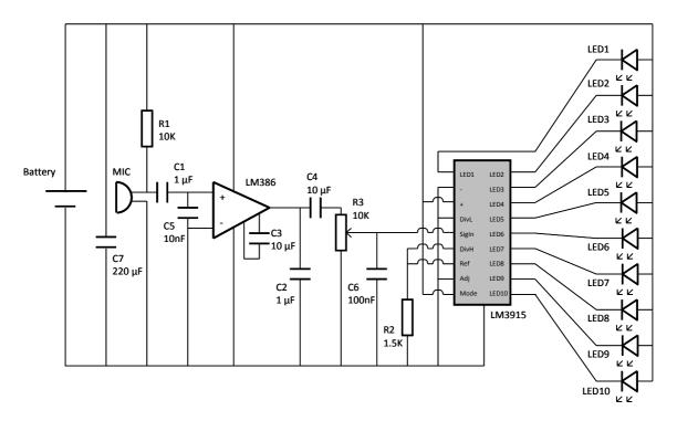
The sound meter circuit uses a microphone to detect sound and then uses a number of LEDs to indicate the how loud the sound is.
