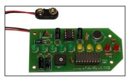
Before you put any components in the board or pick up the soldering iron, just take a look at the Printed Circuit Board (PCB). The components go in the side with the writing on and the solder goes on the side with the tracks and silver pads.
