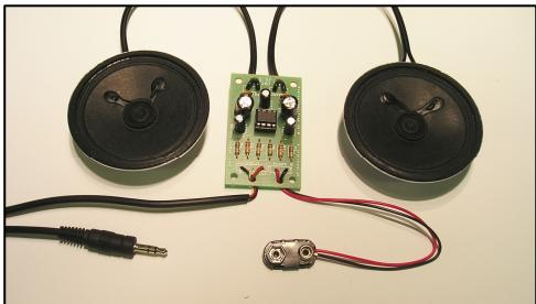
Before you put any components in the board or pick up the soldering iron, just take a look at the Printed Circuit Board (PCB). The components go in the side with the writing on and the solder goes on the side with the tracks and silver pads.
