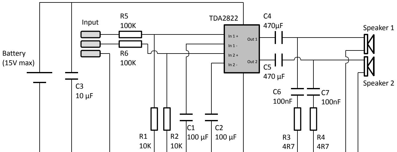
At the centre of the circuit is an audio amplifier Integrated Circuit or IC. Inside the IC are lots of transistors, which are connected together to allow the small input signal to be amplified into a more powerful output that can drive a speaker.
