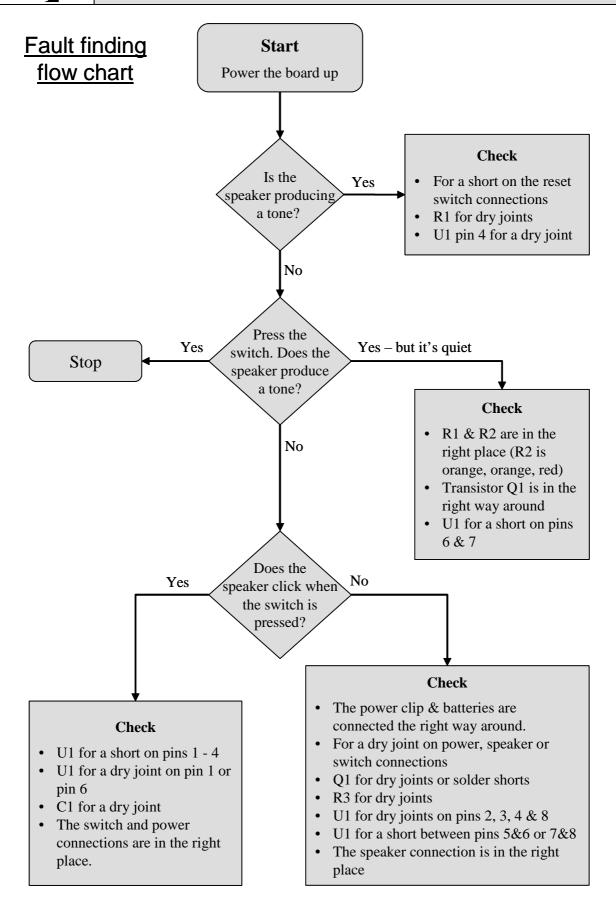
Please note: This fault finding diagram is based upon using an  $8\Omega$  speaker to test the circuit. Alternatively an oscilloscope connected to the logic output could be used.
