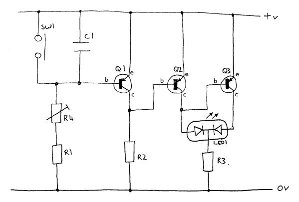
When the power is connected to the circuit, capacitor C1 will start to fill. As this fills with charge the voltage across it gets bigger. The variable resistor R4 controls the speed at which the capacitor fills.
