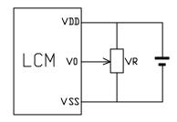
$V_{DD^{\sim}}V_0$ : LCD Driving voltage
