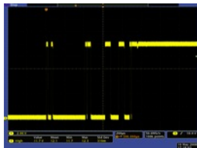
Oscilloscope capture of the output voltage of a large mechanical switch as it bounces.
