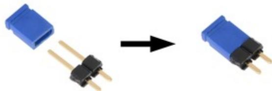
**Connecting a 1×2-pin male header to a blue shorting block makes a tool that can be used to activate the learning mode on the Pololu RC Switch with Relay.**
