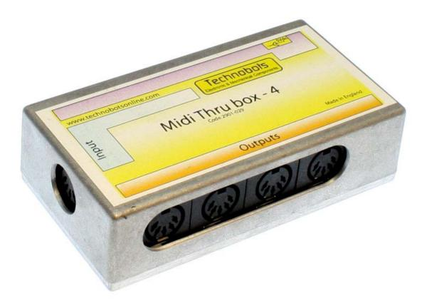
The MIDI Thru box – 4 can drive up to 4 slave MIDI devices from the one input signal. These thru boxes are very straightforward to use, simply plug a lead in from the master MIDI signal out (or thru if needed) to the thru box input using a standard 5-pin 180° DIN plug lead. Connect the thru box outputs to the IN sockets on the MIDI slave units again using standard 5-pin 180° DIN plug leads.
