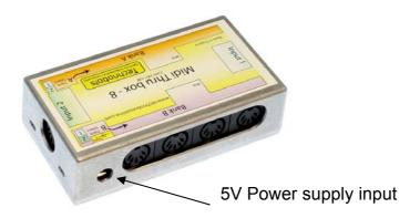
That's it, you are ready to go. The thru box draws very little power just 10-30mA and the adaptor is also very efficient so energy consumption is negligible. Please note that the power supply must be 5V dc regulated, damage to the thru box electronics may occur if an incorrect voltage is used.
