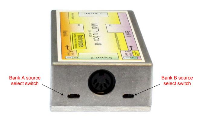
Viewing from the end, moving the switch to the left selects input 1, to the right input 2. To move the switch, use the tip of a pen or small screwdriver etc..
