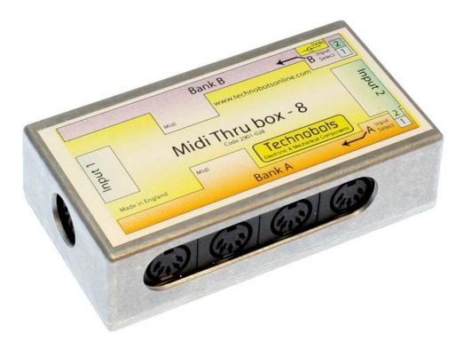
The MIDI Thru box -8 can drive up to 8 slave MIDI devices from the one input signal or two banks of 4 slave MIDI devices from 2 inputs. The choice is made using the recessed switches located at input 2 end of the Thru box.
